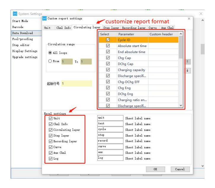
4. Modify circular statistic method, Charge/discharge efficiency, platform voltage, or keep defaut setting
